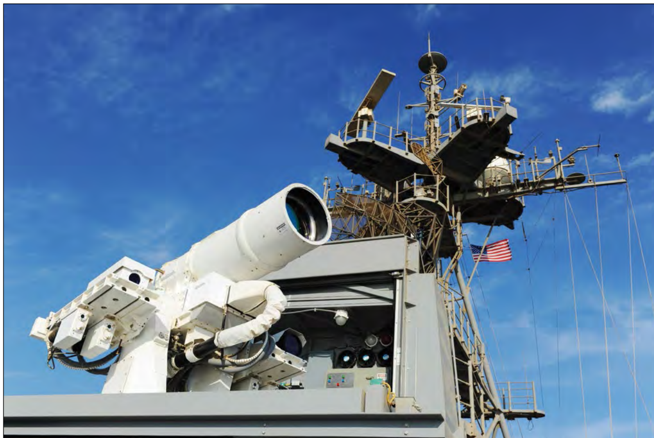
AN/SEQ-3 laser system on board USS Ponce .
