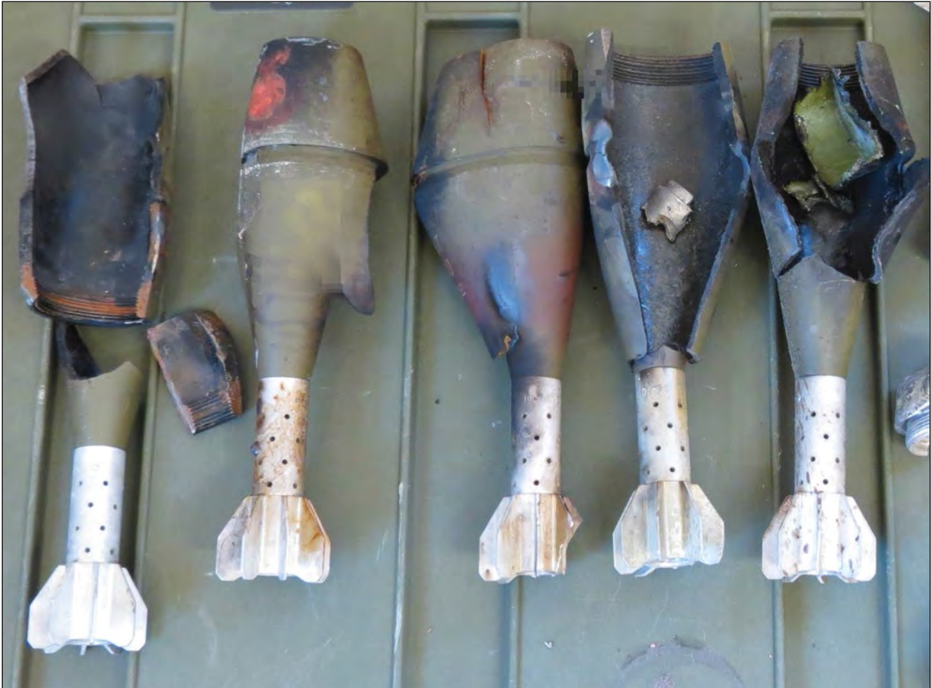
Mortar rounds neutralized using a HEL.
